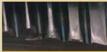
Edge chipping and wear at the chamfer.
