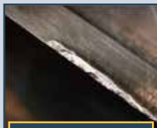
Comp. A (Severe wear, chipping)
